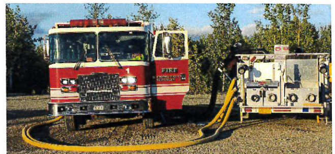
Pumper service testing on Engine 92
