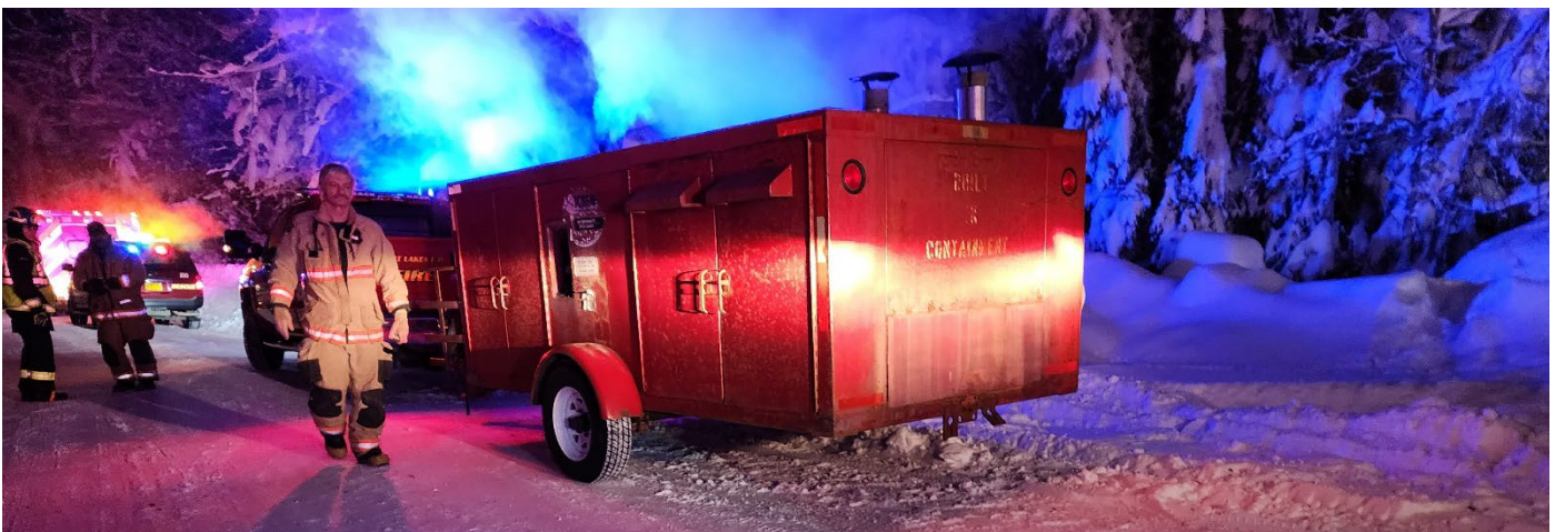
Trailer heater to thaw crews and equipment in extreme freezing weather
